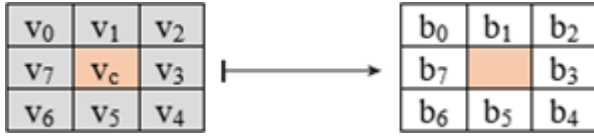
Figure 5. Illustration of first and second step of LBP generation
